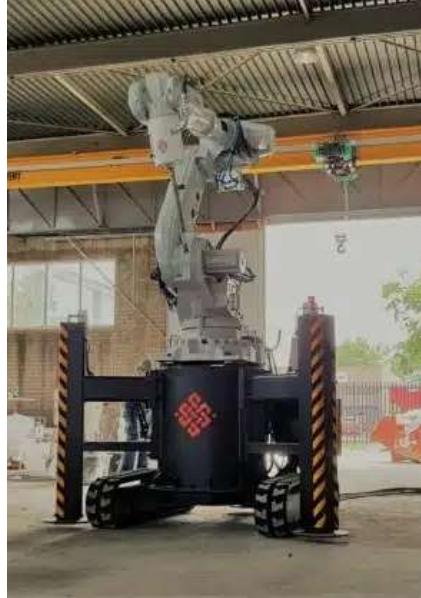
Figure 3.6 Robotic crawler 3DCP (image credit Cybe Construction)
