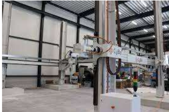
Figure 3.8 Gantry 3DCP (image credit Cybe Construction)
