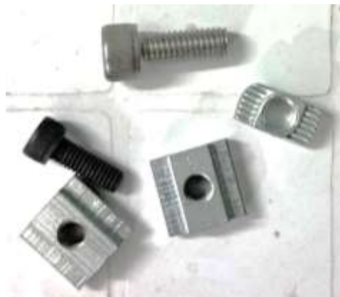
Figure 3.16 Sliding T-Nut and Allen Bolt
