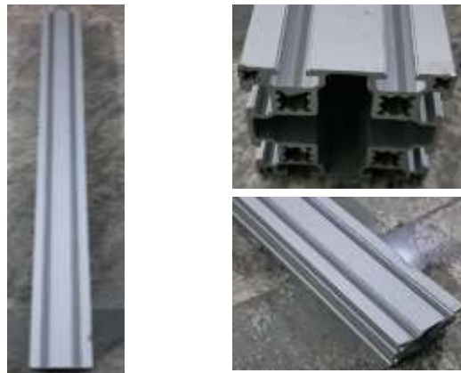
Fig 3.13 Structural Frame (Aluminium Extrusions)
