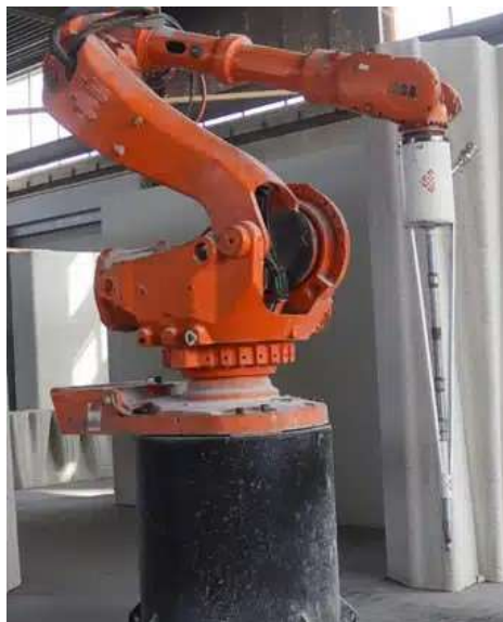
Figure 3.5 Fixed Robot 3DCP (image credit Cybe Construction)
