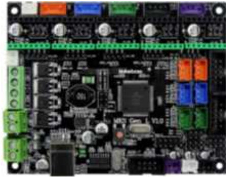
Figure 3.20 MKS Circuit Board image credit www.makerbase.store
