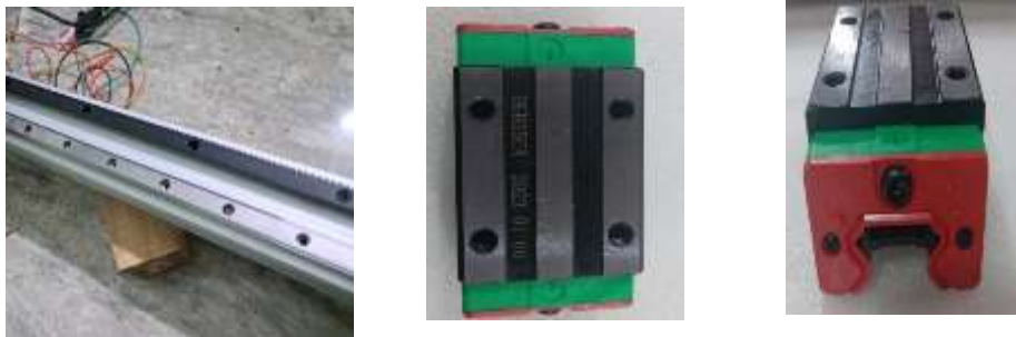
Fig 3.14 Linear Guide Rail and Sliding Block
