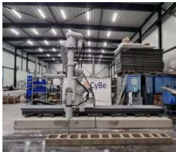
Figure 3.7 Robotic track 3DCP (image credit Cybe Construction)
